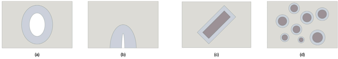
Fig. 3. Cloaking of an elliptic hole (a), an elliptic cut (b), a rectangular inhomogeneity (c), and randomly distributed circular inhomogeneities (d). The blue color shows the cloak C.
